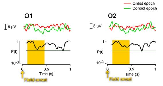
The EEG recorded from the 2 occipital electrodes is shown at the top. Each of the points in the region where the evoked potential was expected was compared with its corresponding control by means of the t test. As you can see, none of the tests were statistically significant, indicating that the presence of an evoked potential was not detected in the method of time-averaging.
