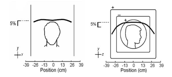
A magnetic field that was homogeneous to within 5% was applied using a pair of 3 coils. The coils were designed using a commercial software program, and field uniformity was verified by measurements using a fluxgate magnetometer.
