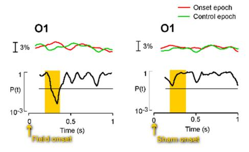
This is the corresponding result using %R. You can see than an evoked potential was detected in the expected time interval when the data was analyzed using an analytical method that allows for the presence of nonlinear determinism. The sham-field analysis was negative, as expected. This result was obtained on a particular patient using the EEG measured at O1.
